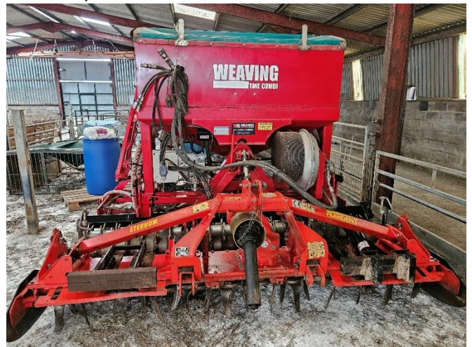
Weaving 3m Combination Drill Tine Drill, Small Seed Kit, Frandent Power Harrow, Radar Speed Sensor.
