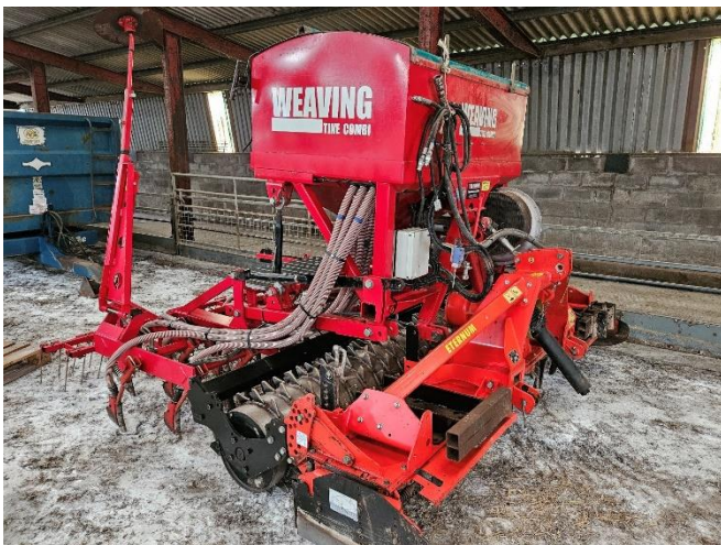
Weaving 3m Combination Drill Tine Drill, Small Seed Kit, Frandent Power Harrow, Radar Speed Sensor.
